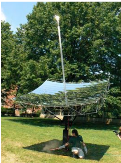
Team member Matt Ritter shows steam coming out of the return hose after it forms in the coil above the solar dish.
