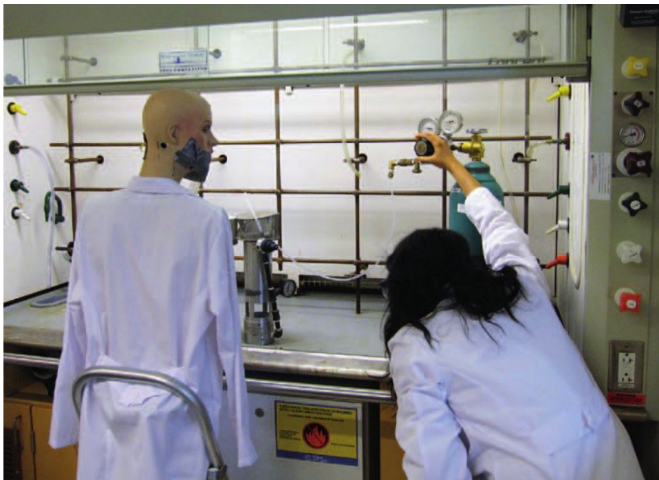
UROP student Evelyn Zuniga adjusts the release of the tracer gas substitute into the fume hood as “Betty” the test mannequin looks on. An air intake at Betty’s mouth and nose will simulate the breathing of a researcher to test for the possible presence of the tracer gas in front of the fume hood.
