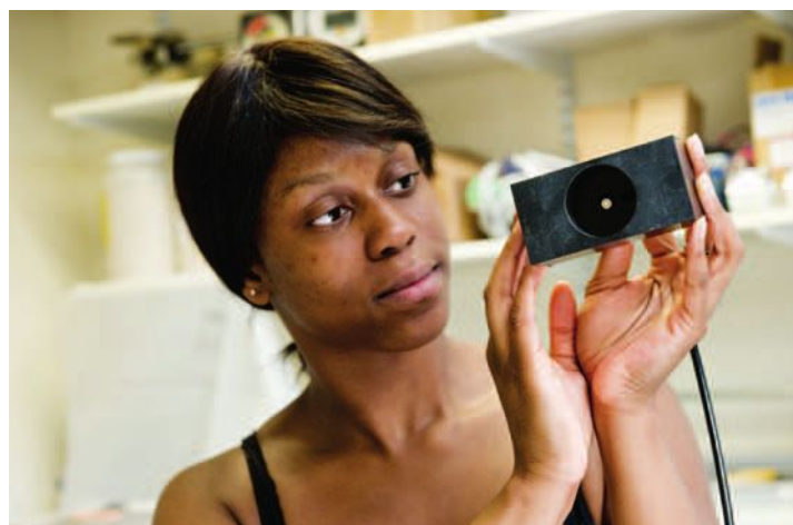
Jennifer Hammond '12 of mechanical engineering demonstrates a device that measures the reflectivity of a surface. Using the device, she has been examining how dust or sand deposited on reflective surfaces can reduce the efficiency of a parabolic solar trough in the desert.
