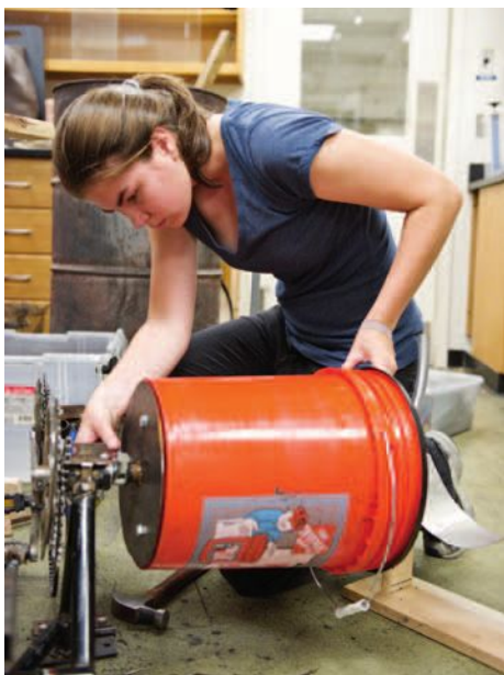
Rachel Dias Carlson '14, of mechanical engineering, attaches a charcoal agglomeration prototype to her pedal-power setup. Her UROP aimed to develop new machinery that can carbonize and briquette agricultural waste at the same rate at which the waste is produced in developing countries.
