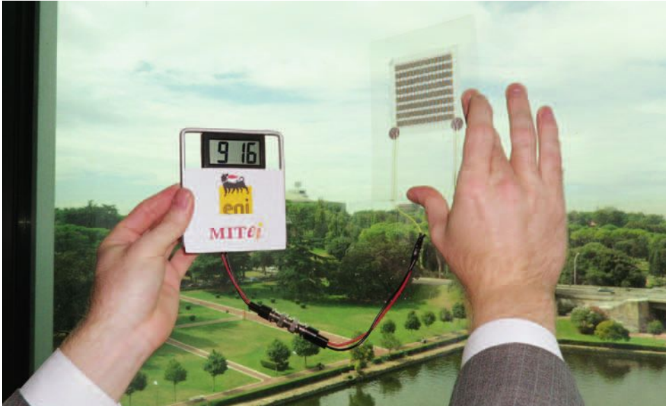
The prototype array shown here contains 250 PV cells on a 7 cm by 7 cm piece of paper laminated in plastic. In natural light on a cloudy day, it generates 50 volts—enough to power the LCD clock display in the photo.
