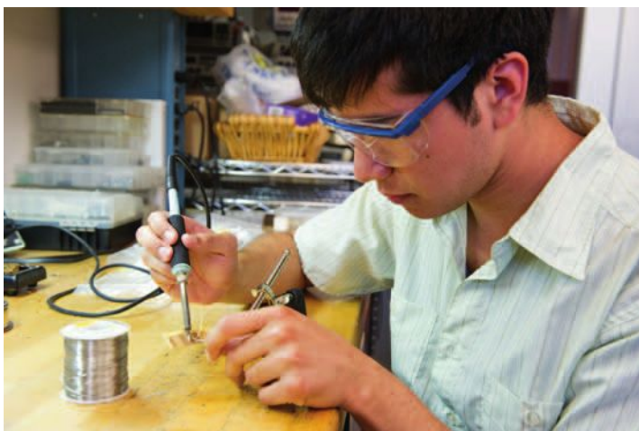
Martin Lozano '12, of mechanical engineering, solders components onto a circuit board to control an underwater robot. His summer UROP focused on creating a compact, submersible robot to inspect the underground pipes of nuclear power plants internally—a task that normally requires unearthing the pipes and risking exposure to potentially dangerous levels of radiation. Lozano also programmed the robot's control code and designed a graphical user interface.
