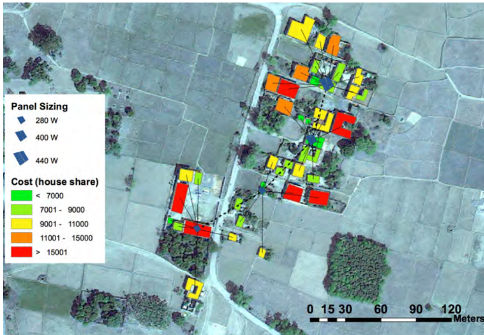
This GridForm model of a village in Bihar, India, shows the optimal layout of hardware for the load profiles of the community. Each building, color-coded by the cost (in Indian rupees) of supplying electricity to that structure, is wired to a central generation/storage node (solid lines), and the nodes are connected to each other (dotted lines).
