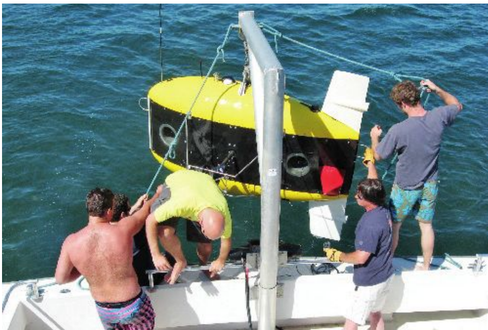
MIT researchers launch Odyssey IV for sea trials off Woods Hole, Massachusetts. The vehicle weighs 450 kg (1,000 lb). Once in the water, it can cruise at speeds of up to 1.4 meters per second or can hover in place.
