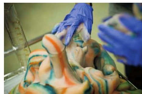
Top: An eruption of foam illustrates the importance of surface tension in an exothermic (energy-releasing) reaction during a 3.012 demo called elephant toothpaste. In this reaction, hydrogen peroxide (mixed with a bit of soap) is catalyzed by potassium iodide to become water plus oxygen: 2\text{H}_2\text{O}_2 \rightarrow 2\text{H}_2\text{O} + \text{O}_2 . The small amount of \text{H}_2\text{O}_2 generates a large volume of oxygen, which is trapped by the soapy water to form a rapid outpouring of bubbles. Food coloring was added to the inside of the container to make the foam have the appearance of toothpaste (or a candy cane).
