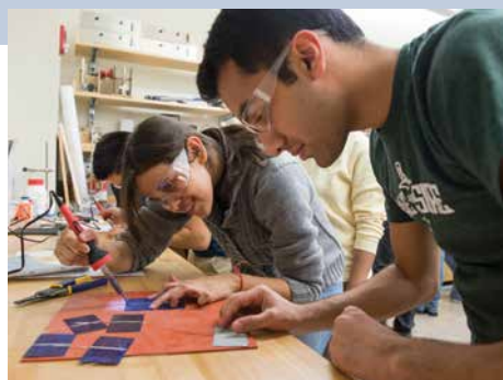
At the IAP workshop, graduate student Neha Mehta (left) and Akhil Nistala '17 solder together solar panels—the first step in assembling their solar-powered cell phone chargers.
