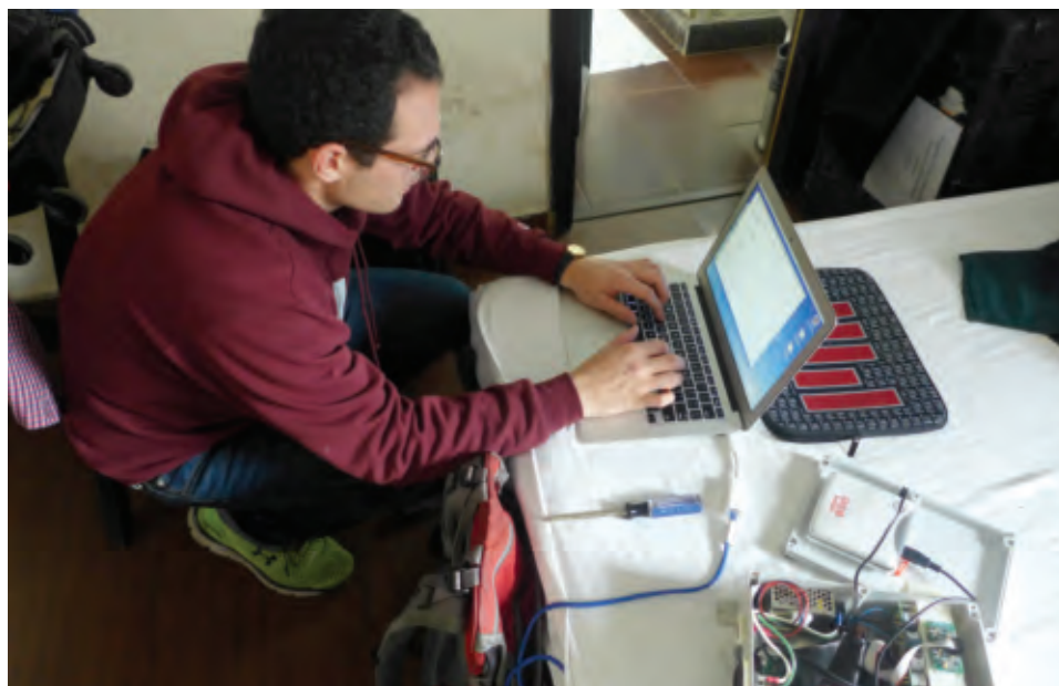
David Hagan, a Tata Fellow and PhD candidate in civil and environmental engineering, is designing and building low-cost sensors that could be deployed in dense networks to monitor air pollution. Here, Hagan makes some last-minute tweaks to his prototype in a hotel room in New Delhi, India.
