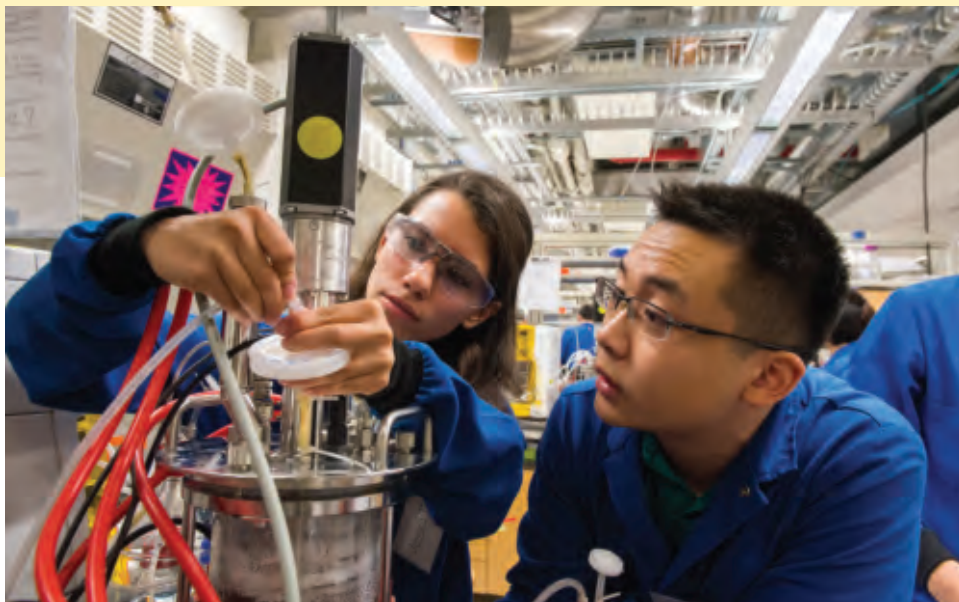
Chemical engineering seniors Jessica Torres (left) and Ruifan Pei work on assembling a bioreactor that uses the genetically engineered bacterium Pseudomonas putida to ferment lignin, a plant waste from cellulosic ethanol, in the process of creating muconic acid.
