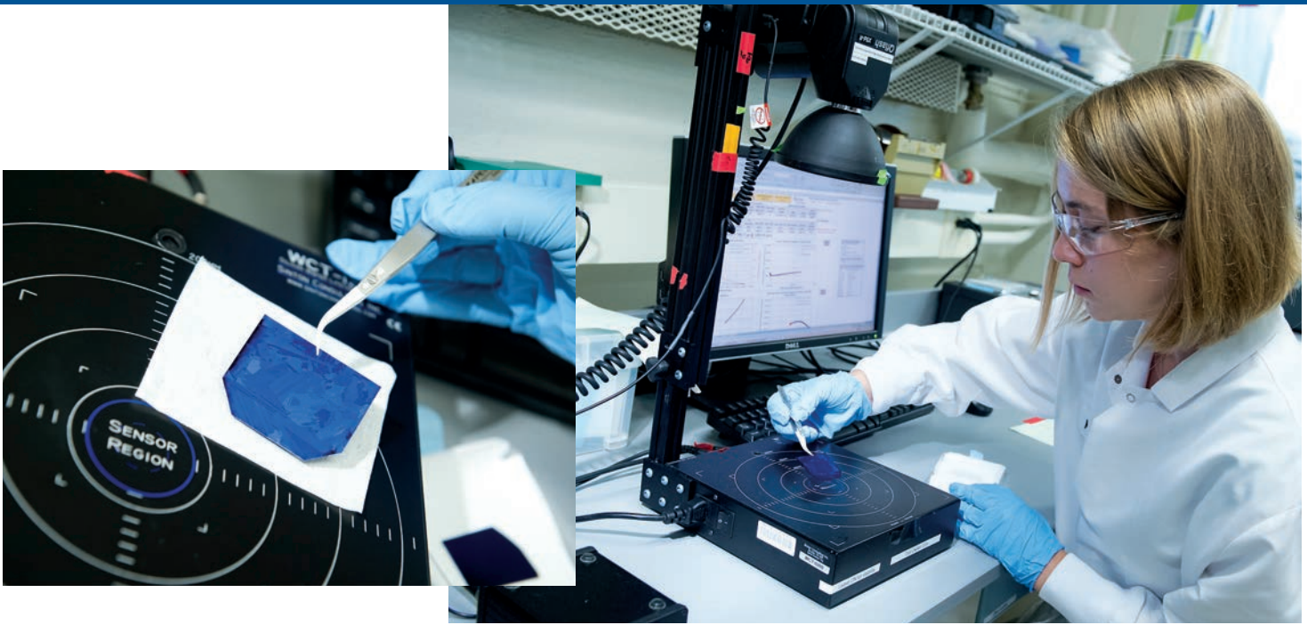
Graduate student Mallory Jensen performs a test to determine the spatially averaged lifetime of excited electrons in a sample silicon wafer. A high-intensity, broadband flash of light excites electrons in the wafer, inducing voltage in a sensor beneath. Inset photo: A close-up of the silicon wafer and the sensor region over which the average is taken.
