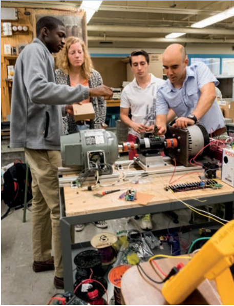
Left to right: UROP students Daniel Vignon '17, Taylor V'Dovec '19, and Juan De Jesus '17, and MITEI postdoc Claudio Vergara adjust a torque and angular speed sensor, which is mounted on a shaft between electrical machines operated as a motor and a generator in their lab-scale model of a power system. The sensor will be used to estimate the electro-mechanical parameters of the machines.
