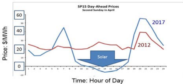
Fig. ES.1. Impact of Added Solar on California Electricity Prices for Second Sunday in April: 2012 and 2017
