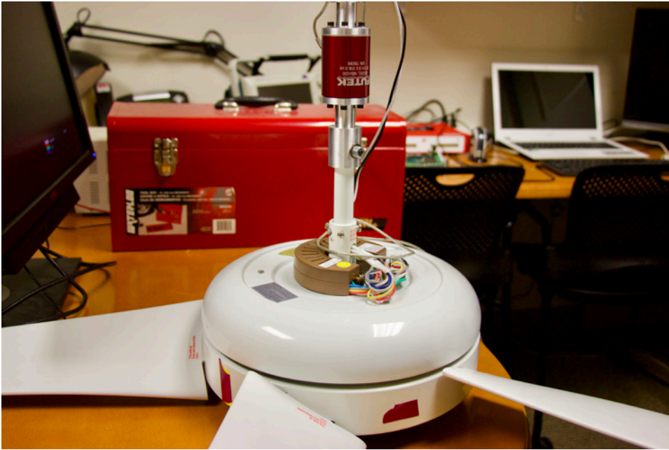
The base shown here contains the motor and the power electronics being tested. Mounted on the pole above are a dynamometer and sensors that measure torque (turning force) and thrust (forward force). Other instruments include a strobotac that monitors the speed at which the fan turns and a hot-wire anemometer that tracks the movement of the air.
