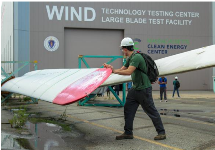
DE FPOP student Moises Trejo tests the flexibility of a wind turbine blade at the WTTC. Photo: Corey Watanabe, MITEI
