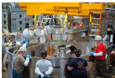
A team of engineers and scientists from CFS and MIT's PSFC lower the superconducting magnet into the test stand in which the magnet was cooled and powered to produce a magnetic field of 20 tesla. Photo: Gretchen Ertl, CFS/MIT-PSFC, 2021
