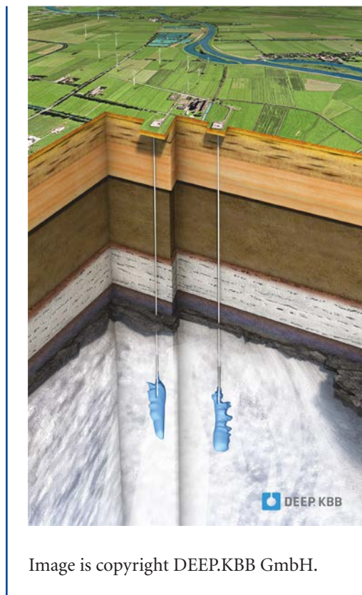
Figure 5.5 Stylized representation of underground salt cavern
