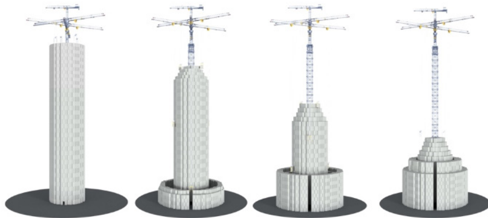
Figure 3.4 A model of the Energy Vault technology
