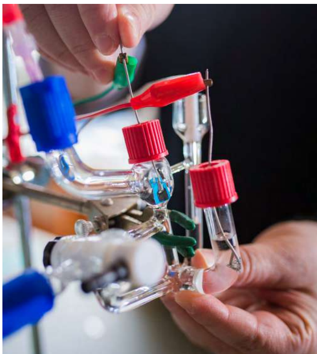
The researchers test and compare the performance of their catalysts using this sealed electrochemical cell. Here, an electrode modified with the catalyst is readied for testing. Once the electrochemical reaction begins, the generated gases will collect in the space above the solution, where they can be sampled and analyzed. Photo: Gretchen Ertl
